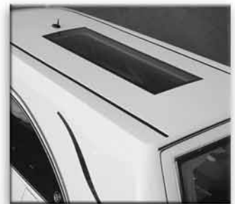
Standard skylight to illuminate casket area.
